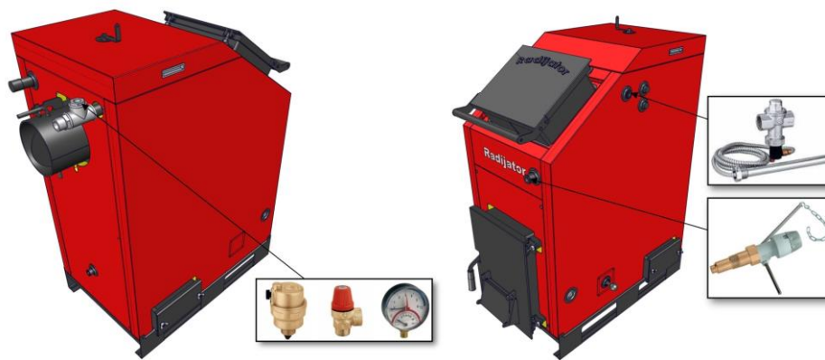
Figure 8. Illustration of placing the safety elements
